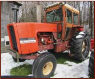
Allis Chalmers Model 7030 Diesel Tractor , Year Around Cab, Dual Hydraulics, 3-Point, 20.8 X 38 Inch Rubber, Unknown Hours
